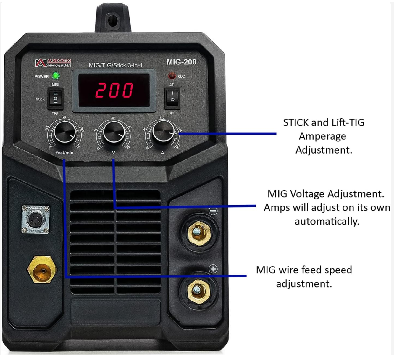
Figure 4.2: Control Panel Overview. This image highlights the key controls: the mode selection switch (MIG/TIG/Stick), the digital display, the STICK and Lift-TIG Amperage Adjustment knob, the MIG Voltage Adjustment knob, and the MIG wire feed speed adjustment knob.
