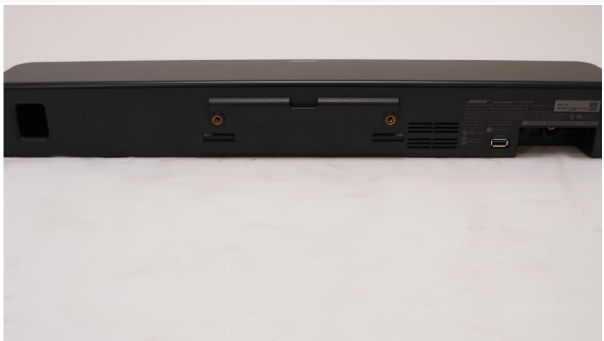
Figure 4: Wall mount points on the soundbar's rear.
