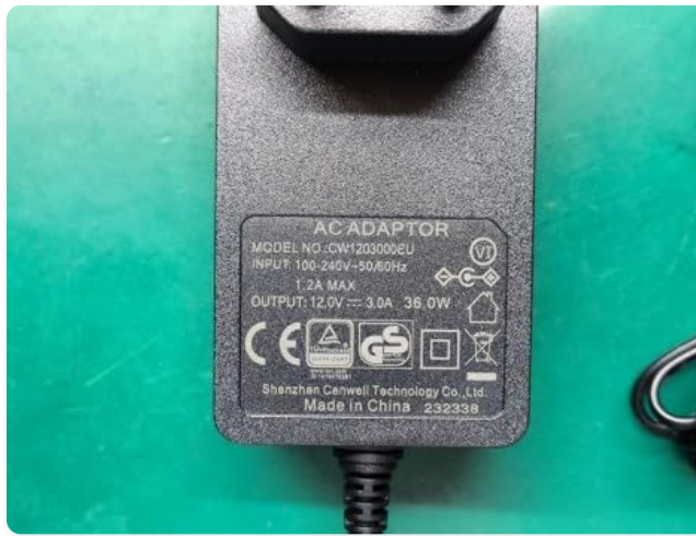
The AC adaptor's label, providing electrical specifications.
