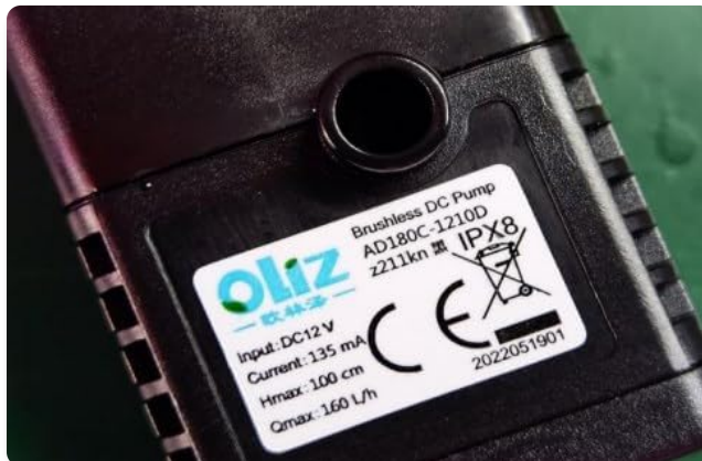
Details of the brushless DC pump, including model and performance metrics.
