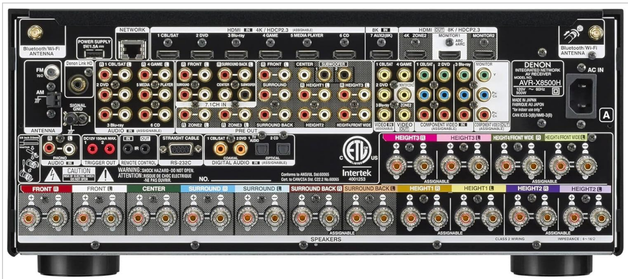
Figure 2.1: Rear panel connections of the Denon AVR-X8500HA.
