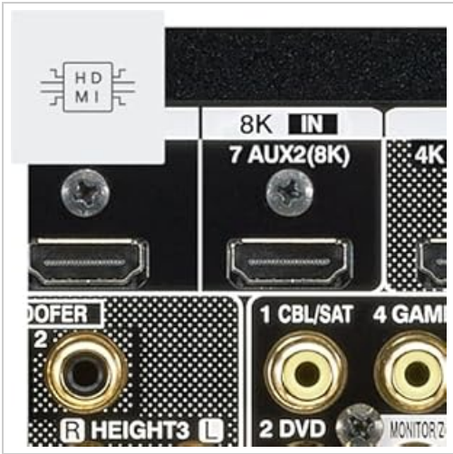
Figure 6.3: HDMI input ports with 8K support.
