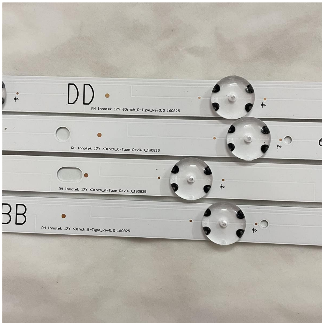
Figure 3.2: A detailed view of an LED strip, highlighting the individual LED lenses and printed part numbers, which should be cross-referenced with your TV's existing strips.
