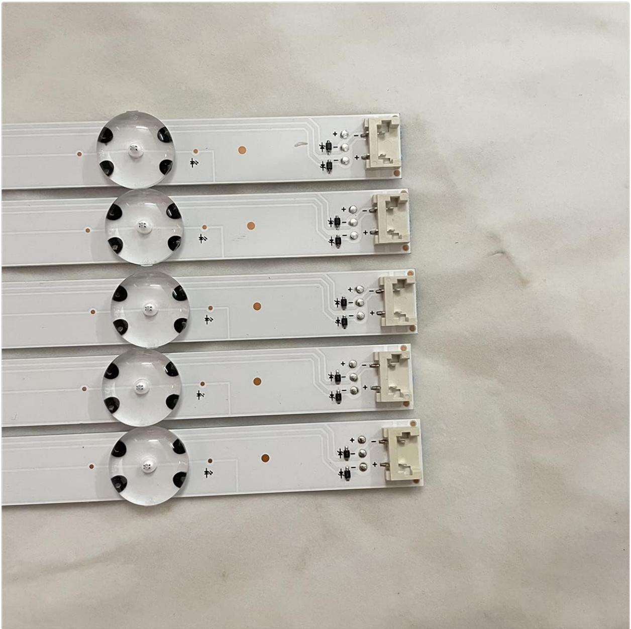
Figure 4.2: A close-up view of the electrical connectors on the LED strips, which must be securely attached to the TV's power board.
