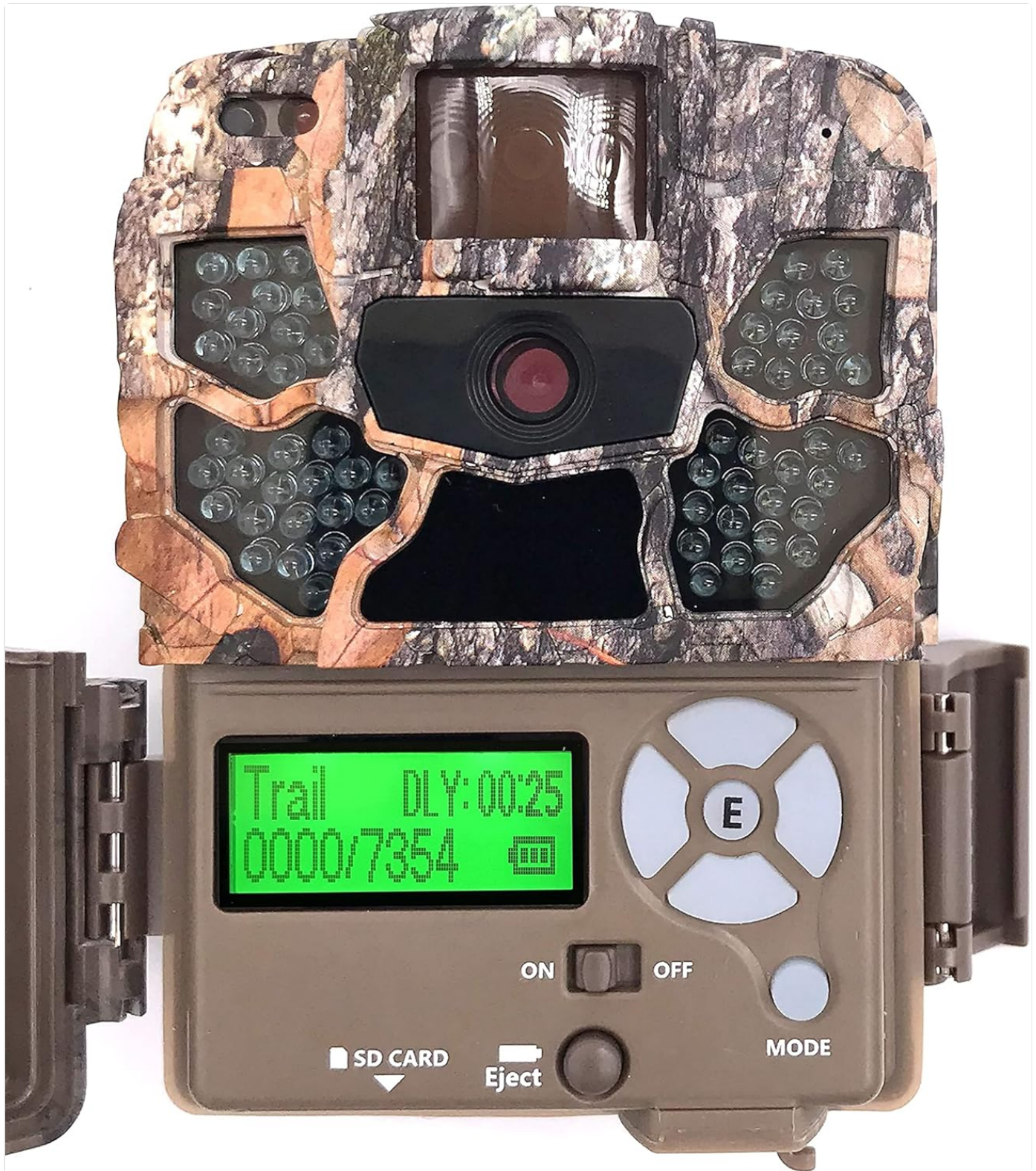
Image: The Browning trail camera with its front panel open, revealing the control screen, navigation buttons, and the SD card slot. The "SD CARD" and "Eject" labels are visible.
