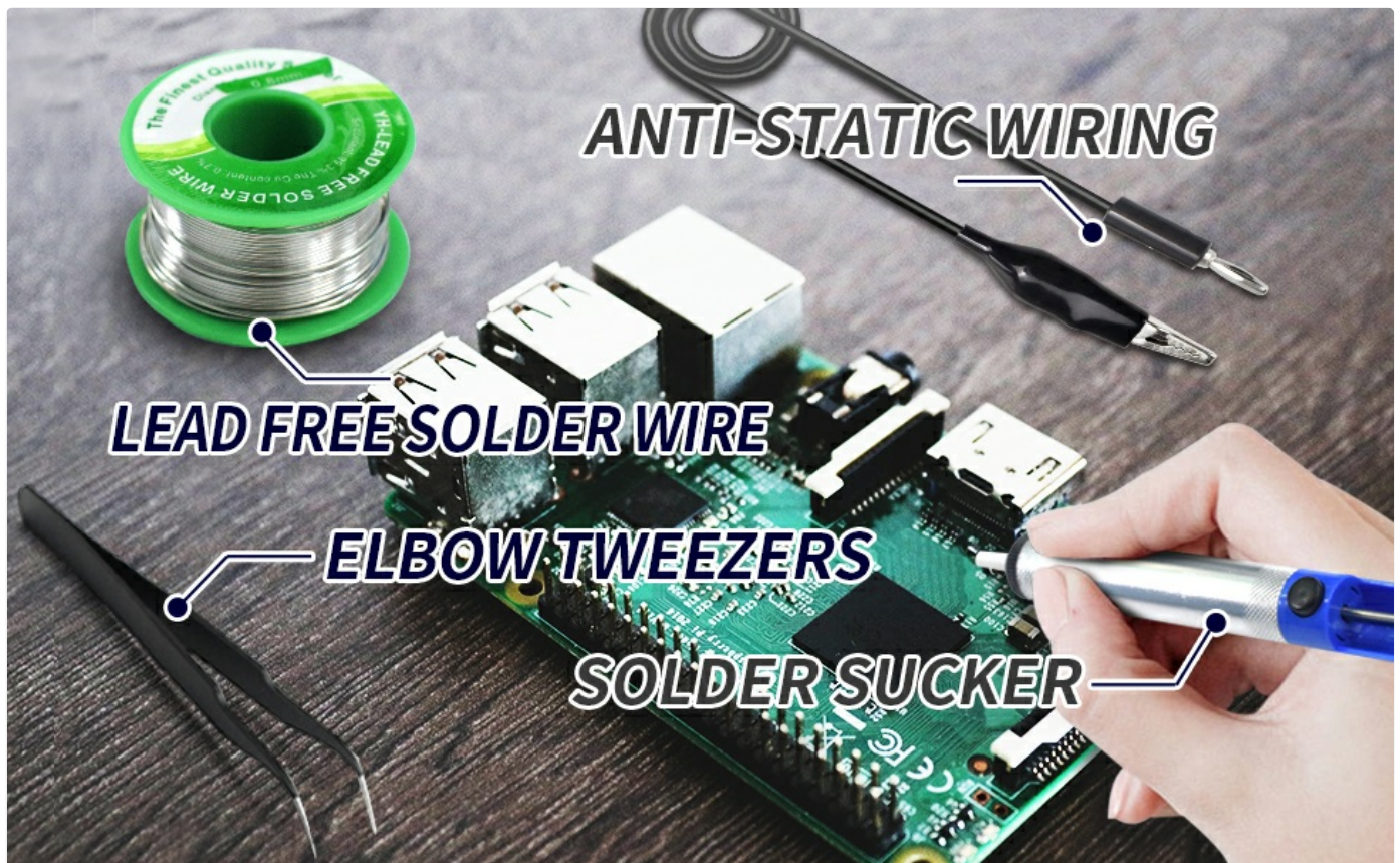
Figure 6.2: Essential soldering accessories such as anti-static wiring, lead-free solder wire, elbow tweezers, and a solder sucker, shown in use with a circuit board.
