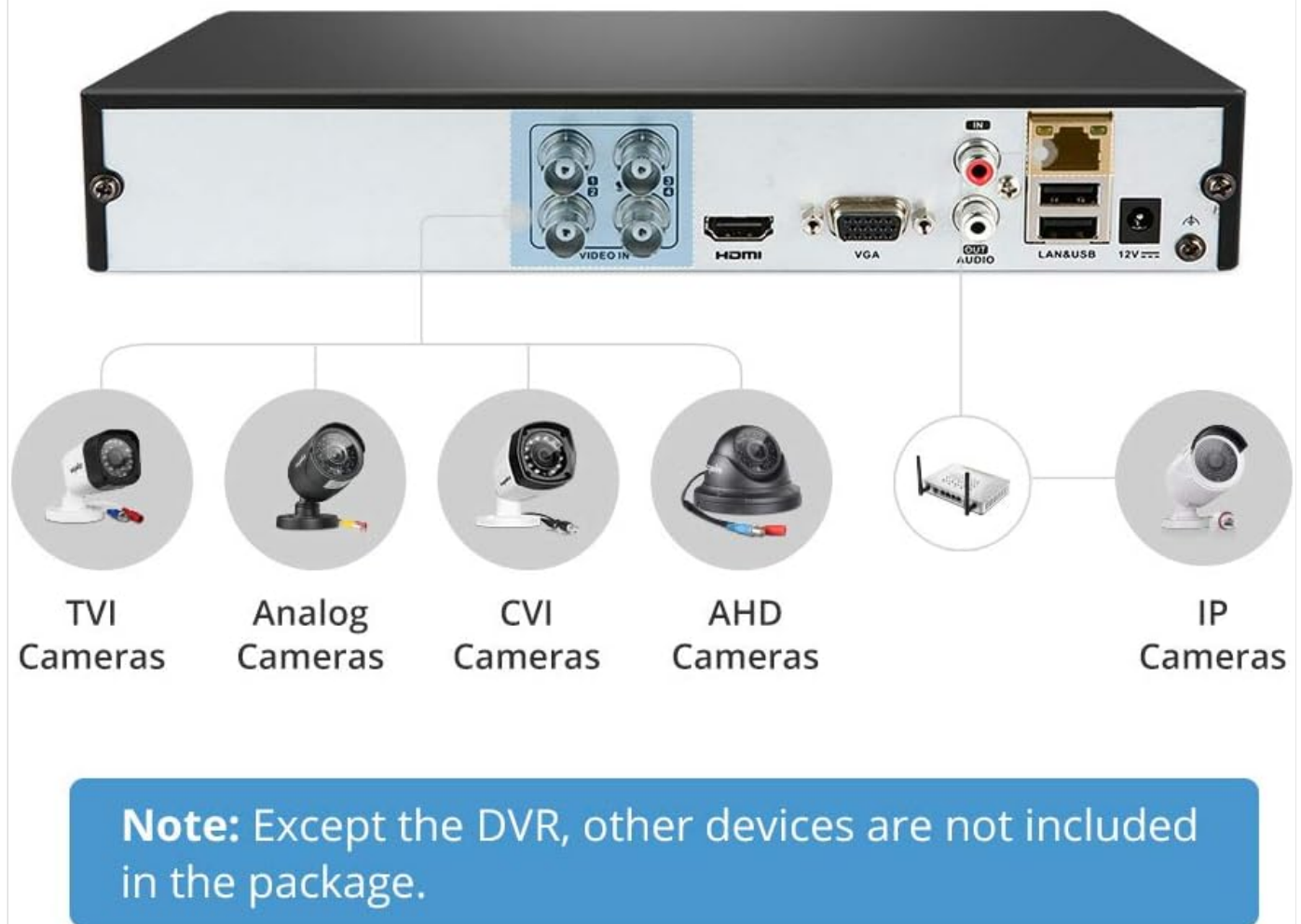
Figure 2.2: Powerful 5-in-1 DVR Compatibility. This image demonstrates the DVR's compatibility with various camera technologies, including TVI, Analog, CVI, AHD, and IP cameras, highlighting its versatility.
