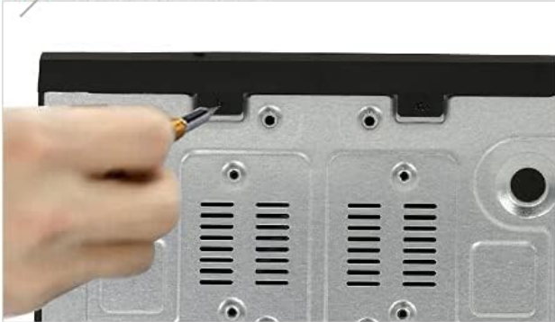
Figure 2.3: HDD Installation Steps. This visual guide shows how to install a hard disk drive (HDD) into the DVR unit, detailing the process of opening the casing, connecting the necessary cables, and securing the drive.
