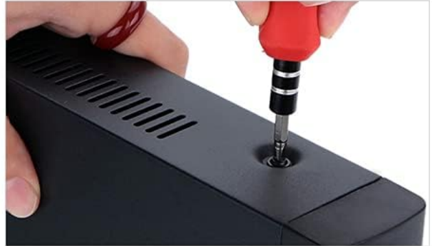
Figure 2.3: HDD Installation Steps. This visual guide shows how to install a hard disk drive (HDD) into the DVR unit, detailing the process of opening the casing, connecting the necessary cables, and securing the drive.
