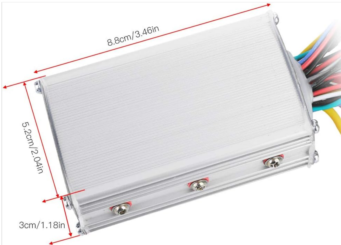
Image: Dimensions of the Yunir Brushless Motor Controller unit.
