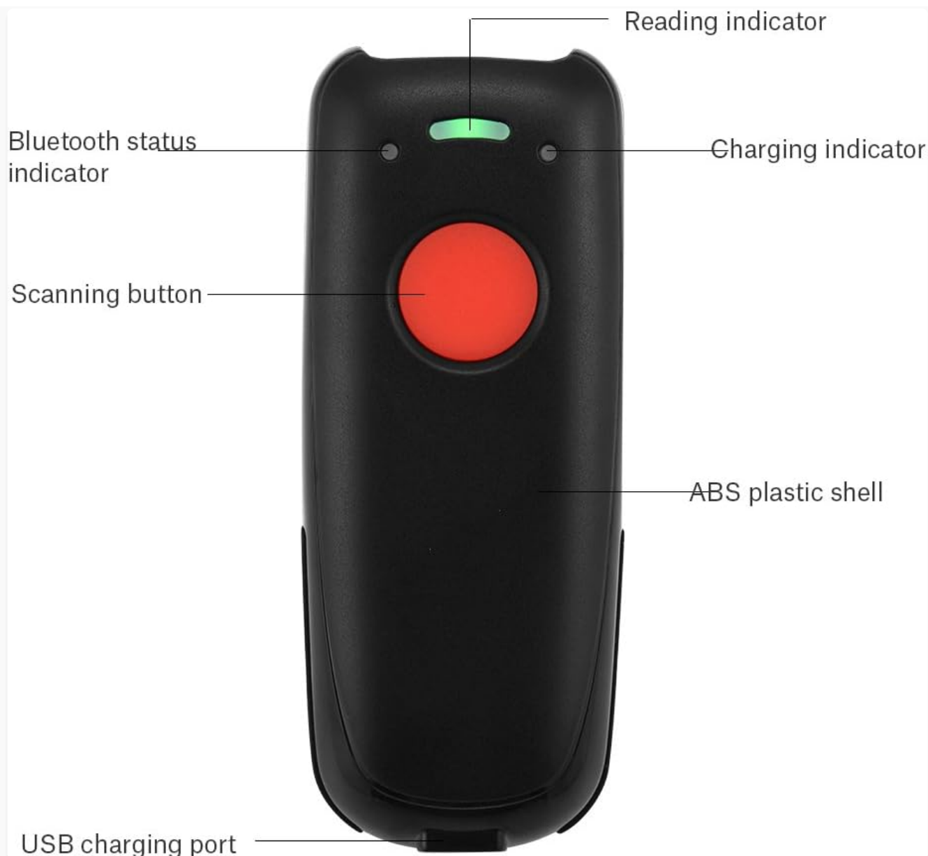
Image 2: A detailed diagram illustrating the various components of the barcode scanner, including the scanning button, Bluetooth status indicator, reading indicator, charging indicator, USB charging port, and ABS plastic shell.
