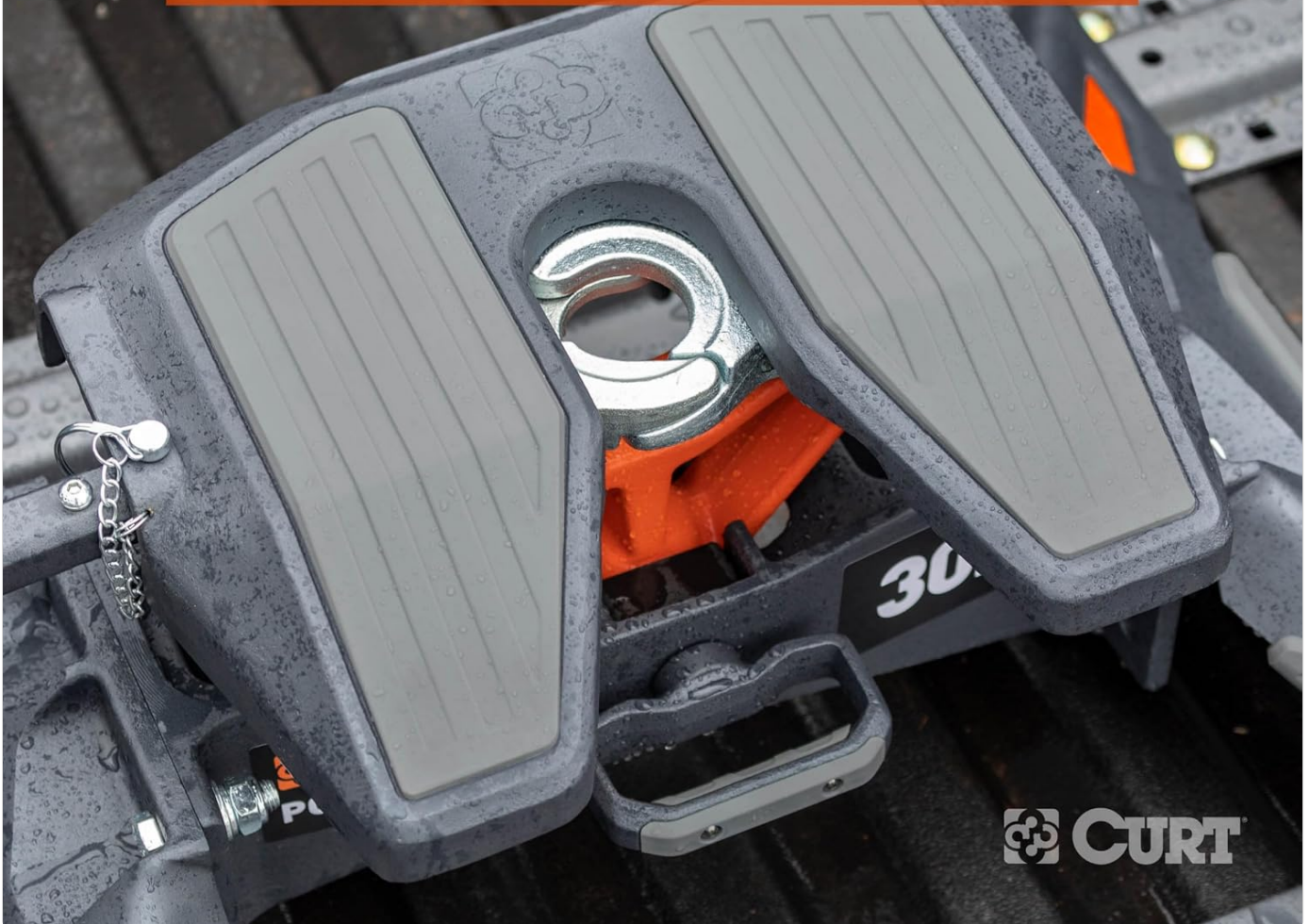
Image: A close-up of the integrated wear plates, designed for smooth operation and reduced maintenance.
