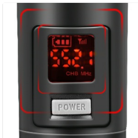
Figure 5: Microphone Display. This image shows a close-up of the microphone's LCD screen, indicating battery status and
