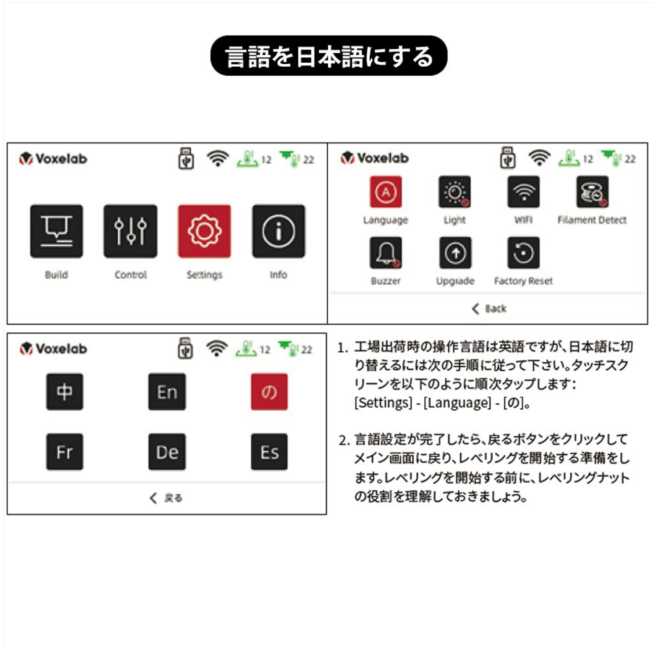
Figure 4: Screenshots of the VOXELAB Aries 3D Printer's touchscreen interface, illustrating how to change the language settings.
