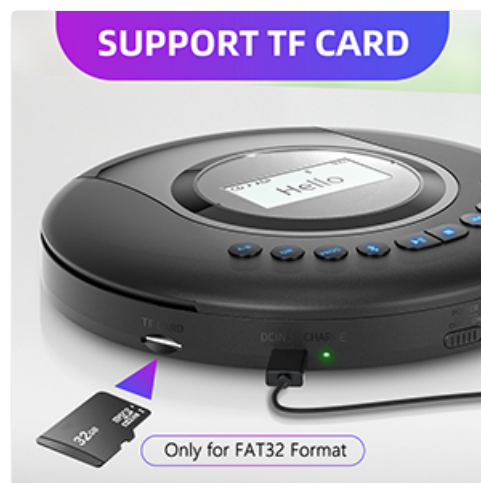
Image 4.3: Location of the TF card slot on the player.
