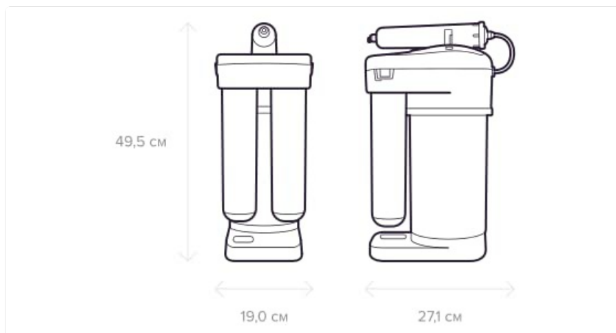
Figure 4: Dimensions of the Aquaphor RO-70S system (L x W x H: 27.1 x 19 x 49.5 cm).
