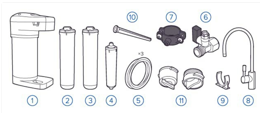
Figure 2: Aquaphor RO-70S System Components.
