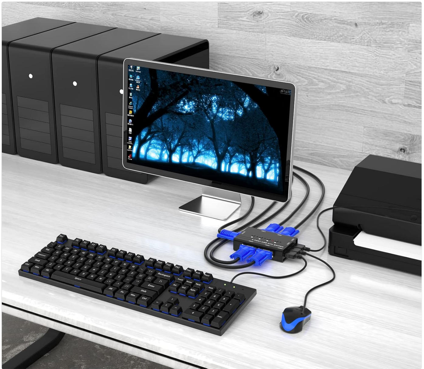
Figure 4.2: Typical Setup. An example of a fully connected KVM switch setup, showing the KVM unit managing multiple computers with a single set of peripherals.
