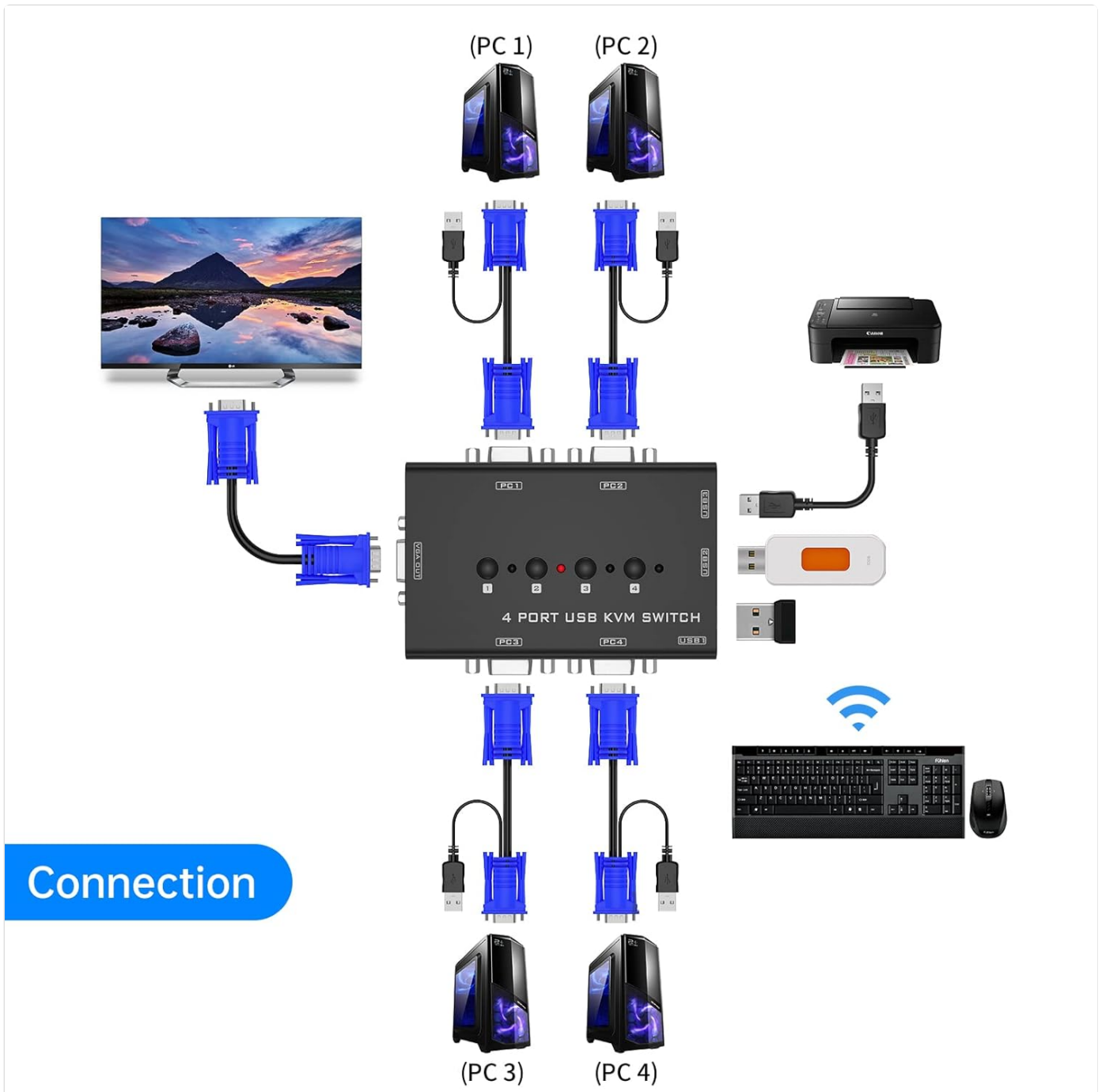
Figure 4.1: Connection Diagram. This diagram illustrates the proper way to connect your computers, monitor, keyboard, mouse, and other USB peripherals to the KVM switch.
