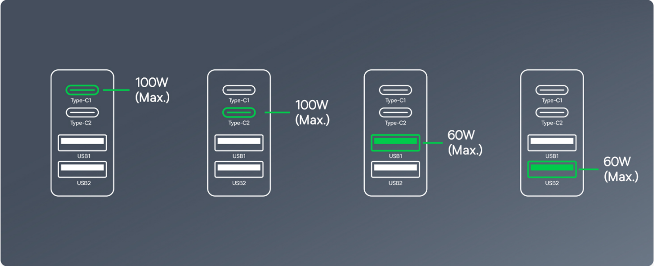
Image: A diagram illustrating various power output combinations when different ports on the Baseus 100W charger are in use, showing maximum wattage per port in different scenarios.
