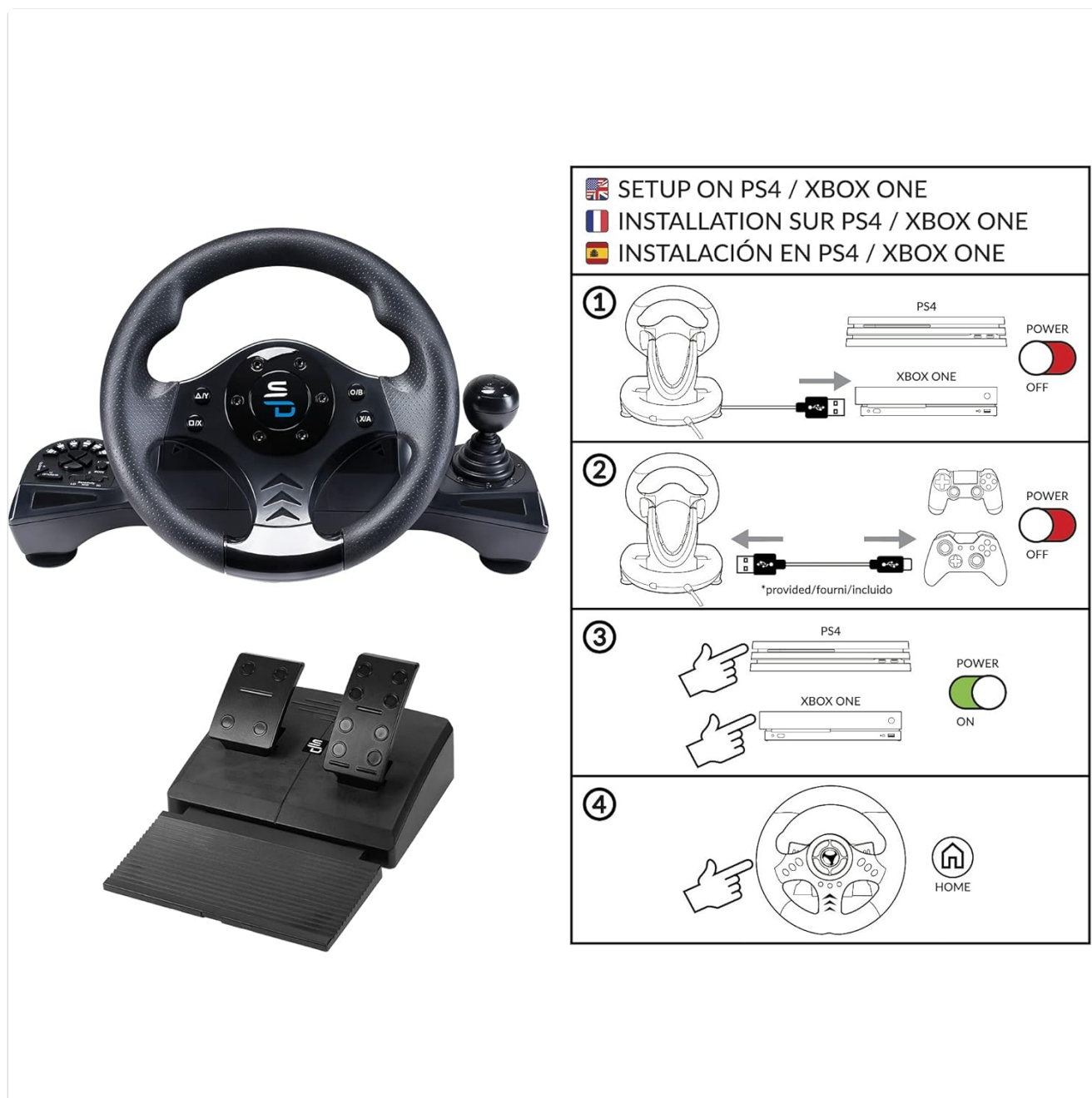
Figure 3: Setup diagram illustrating connections for PS4 and Xbox One consoles, including the requirement to connect an official controller.
