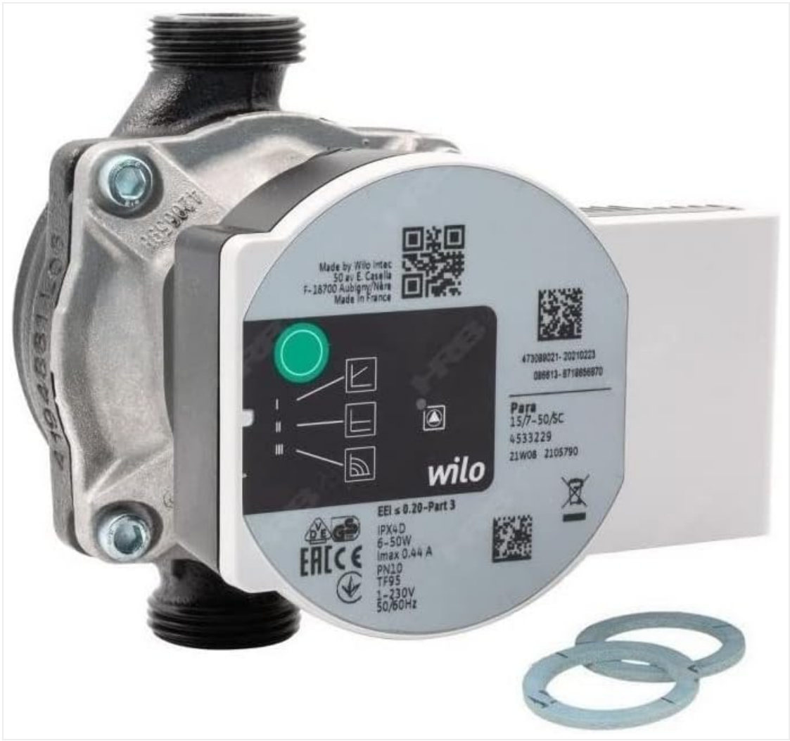
Figure 1: Buderus Para 7M RS 3H Circulator Pump. This image shows the pump from a front-side angle, highlighting its compact design, control panel with a green button and indicator lights, and threaded connections. The label indicates it is made by Wilo Intac in France, with model details 'Para 15/7-50/5C' and technical specifications like EEL \leq 0.20 -Part 3, IPX4D, 6-50W, I_{max} 0.44 A , PN10, TF95, 1-230V, 50/60Hz. Two sealing rings are visible in the foreground.
