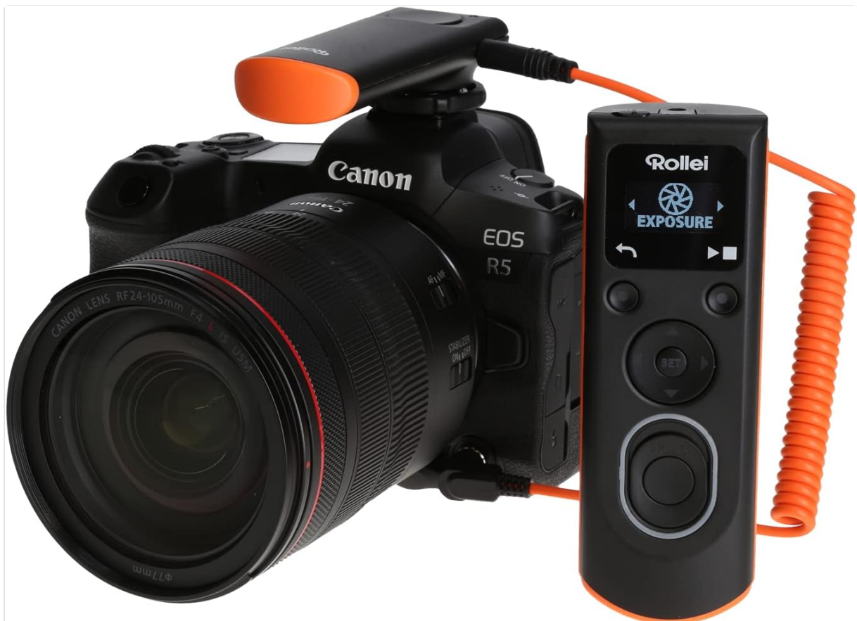
Image 5.1: The remote control display showing the "EXPOSURE" setting, indicating programmable exposure duration for long exposures or time-lapse photography.
