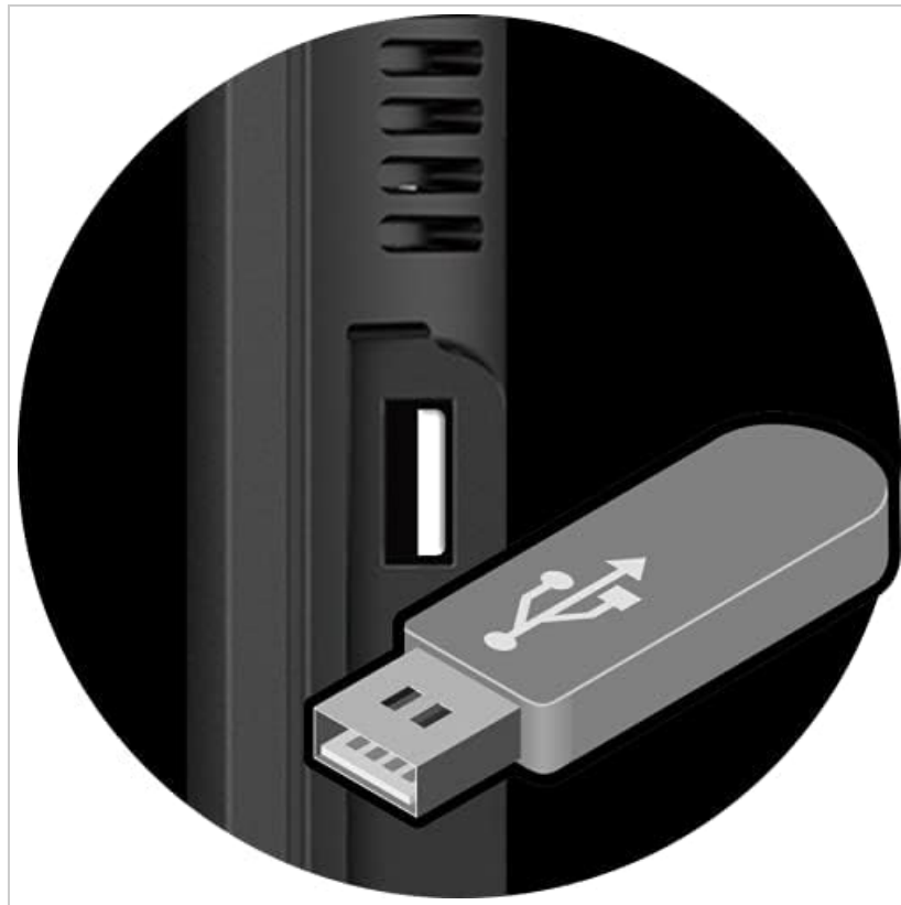
Image 6.1: Detail of the USB port on the efergy Elite-Max display unit, used for data export.
