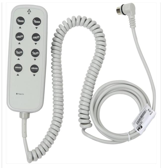
This image displays the complete Okin Dewert 72896 IPROXX2 Handset Remote Control. It shows the gray remote with eight bed adjustment buttons and a 'Power On' indicator, connected to a coiled cable that leads to a 13-pin circular connector.
