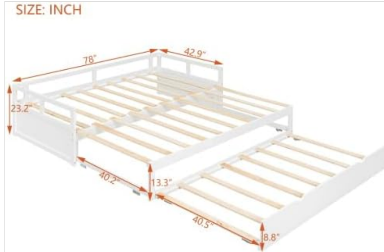
Image: Technical drawing illustrating the dimensions of the daybed in both compact and extended configurations.
