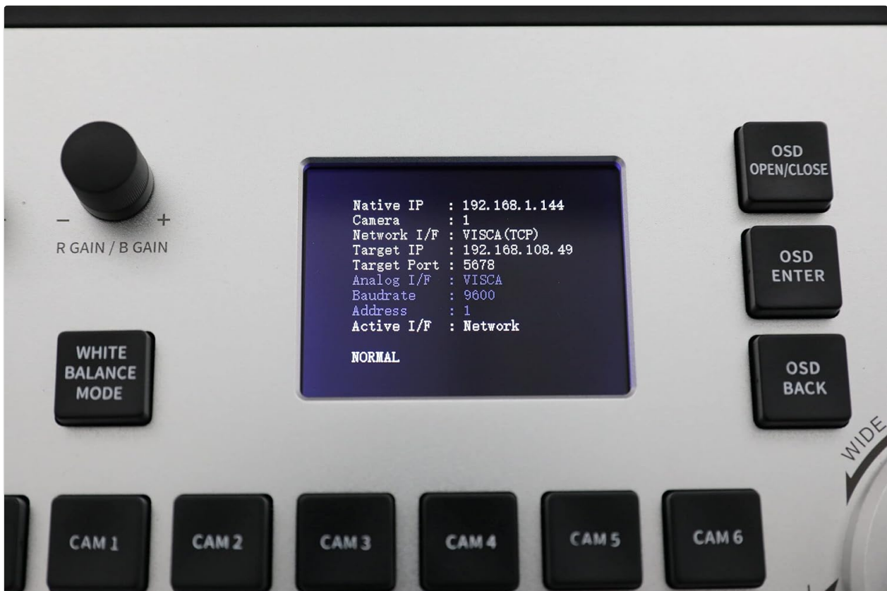
Figure 3.2: The LCD screen showing network interface (Native IP, Target IP, Target Port) and serial interface (Baudrate, Address) settings. This display helps in verifying connectivity and configuration.
