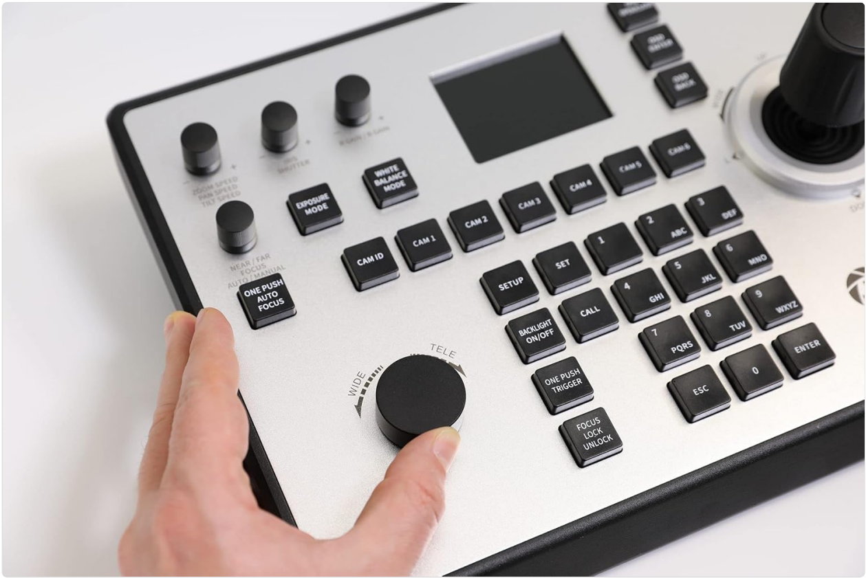
Figure 4.1: A hand demonstrating the use of the zoom knob and the adjacent focus control buttons, illustrating precise camera adjustments.
