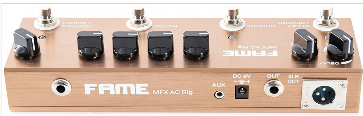
Image 3: Rear view of the Fame MFX AC Rig, showing all connection ports.
