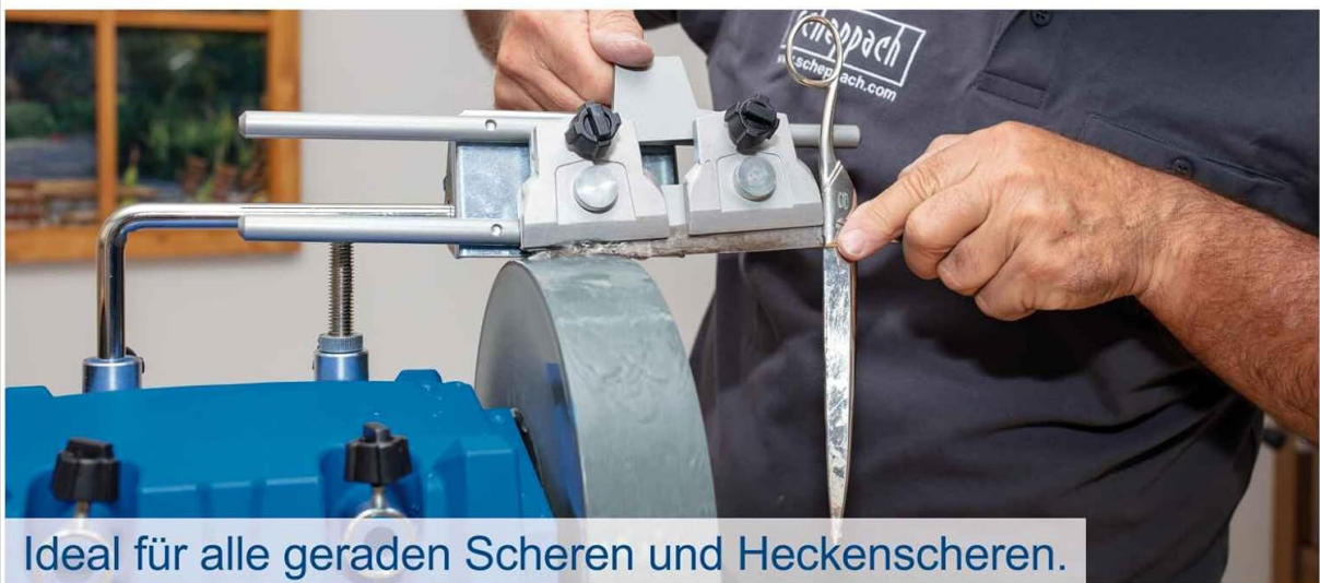
Figure 9: Top image shows sharpening angled edges, pipes, and gouges using an optional jig. Bottom image shows sharpening all straight scissors and hedge trimmers with another optional jig.
