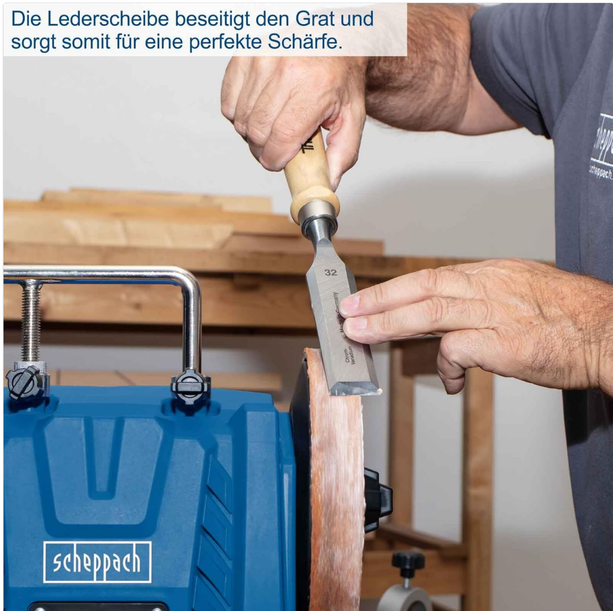
Figure 6: The leather honing wheel removes the burr (grat) from the sharpened edge, ensuring perfect sharpness and a polished finish.
