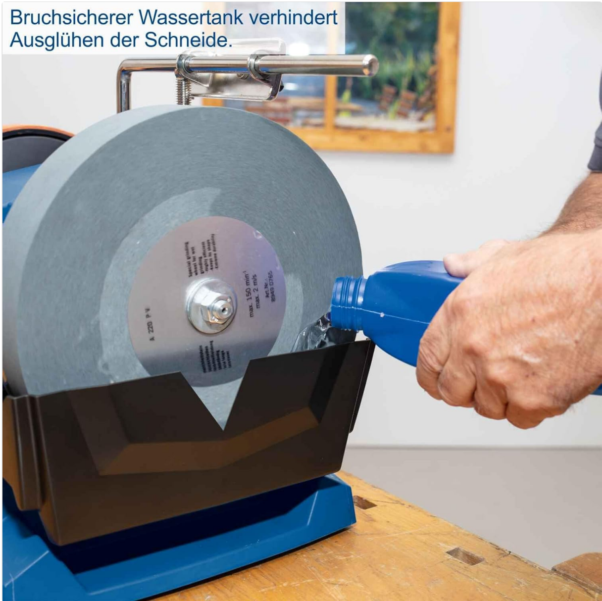
Figure 4: Filling the robust water tank. The tank prevents the blade from overheating during grinding by continuously cooling the whetstone.
