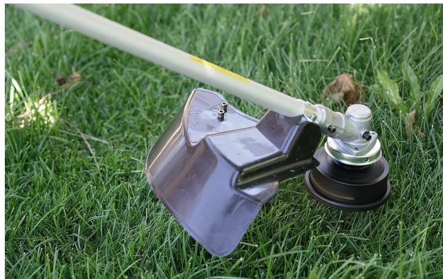
Mount the protective guard over the cutting head area. This guard is crucial for deflecting debris and protecting the user. Ensure it is securely fastened according to the diagram.
