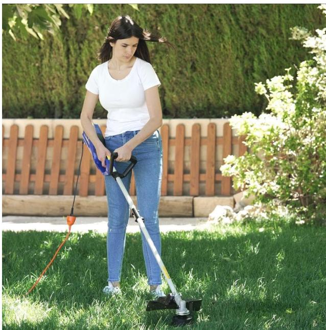
Move the cutting head in a sweeping motion, from side to side, to effectively cut grass and weeds. Maintain a steady pace and avoid forcing the tool through dense vegetation. For best results, cut in small increments.
