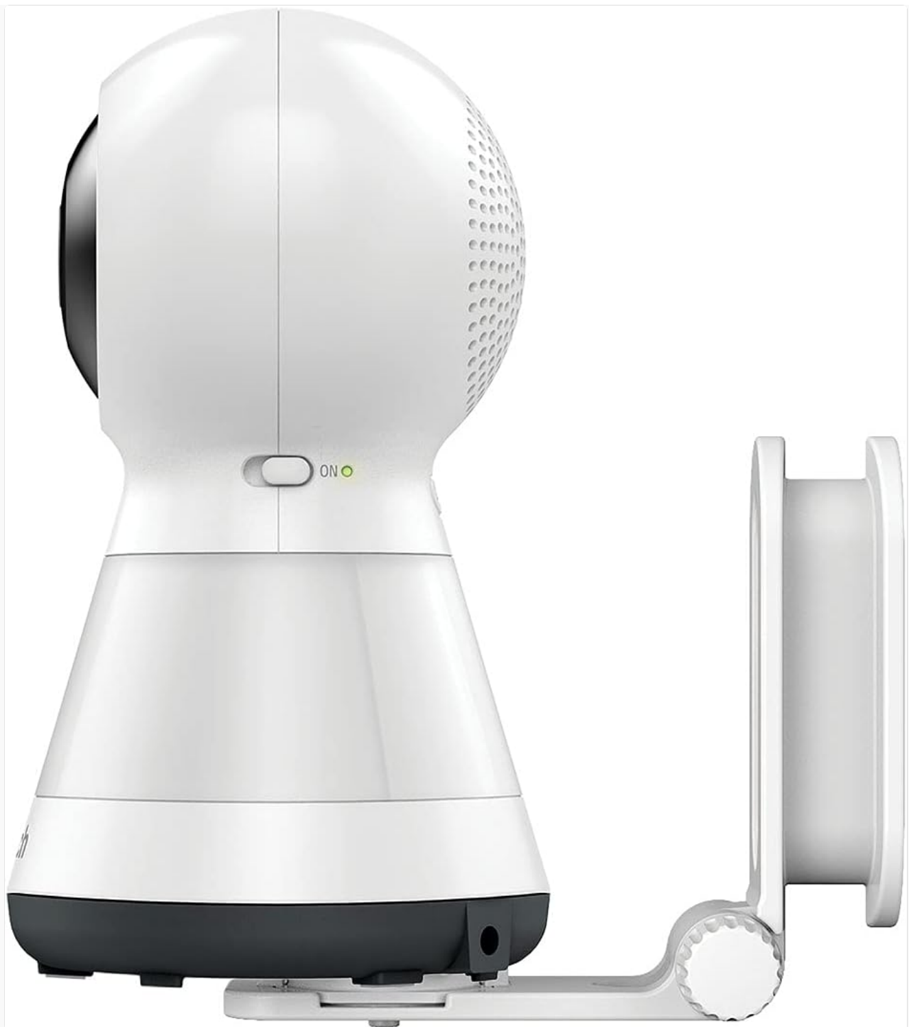
Image: Side view of the VTech VM5255 Baby Unit, illustrating its profile and the optional wall mount bracket.
