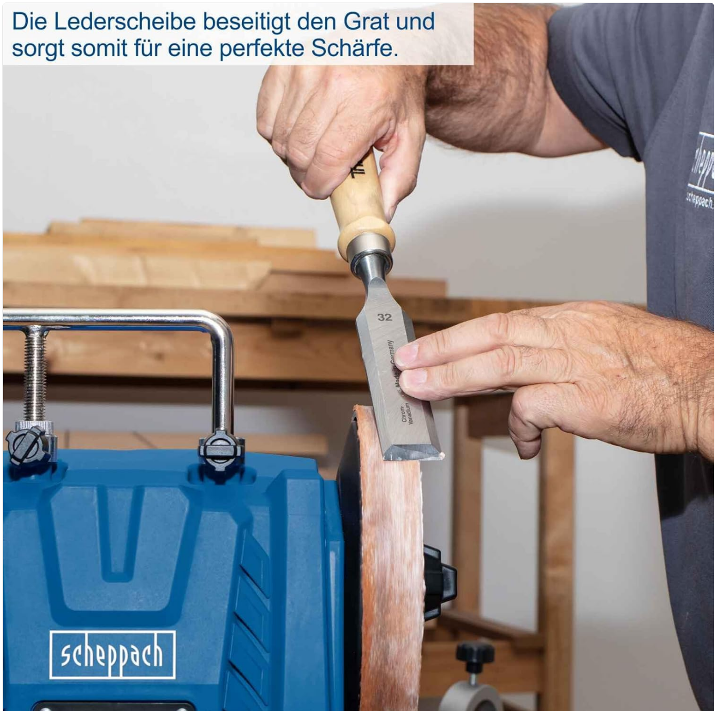
Image: The leather wheel effectively removes burrs, ensuring a perfect sharpness for the tool.
