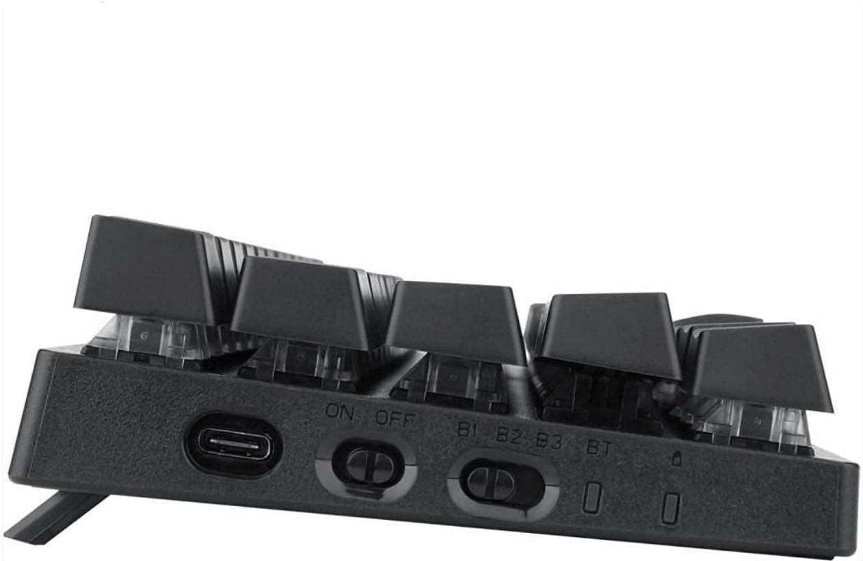
Image: Side view of the T-Dagger T-TGK317 keyboard, showing the 'ON/OFF' switch and dedicated Bluetooth pairing buttons (B1, B2, B3, BT).
