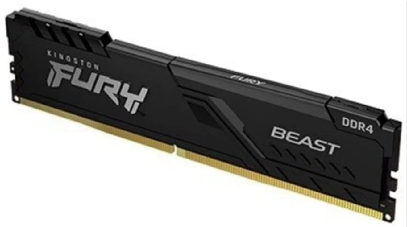
Figure 3.2: Angled view of the Kingston Fury Beast 32GB DDR4 Memory Module, highlighting its low-profile heat spreader.
