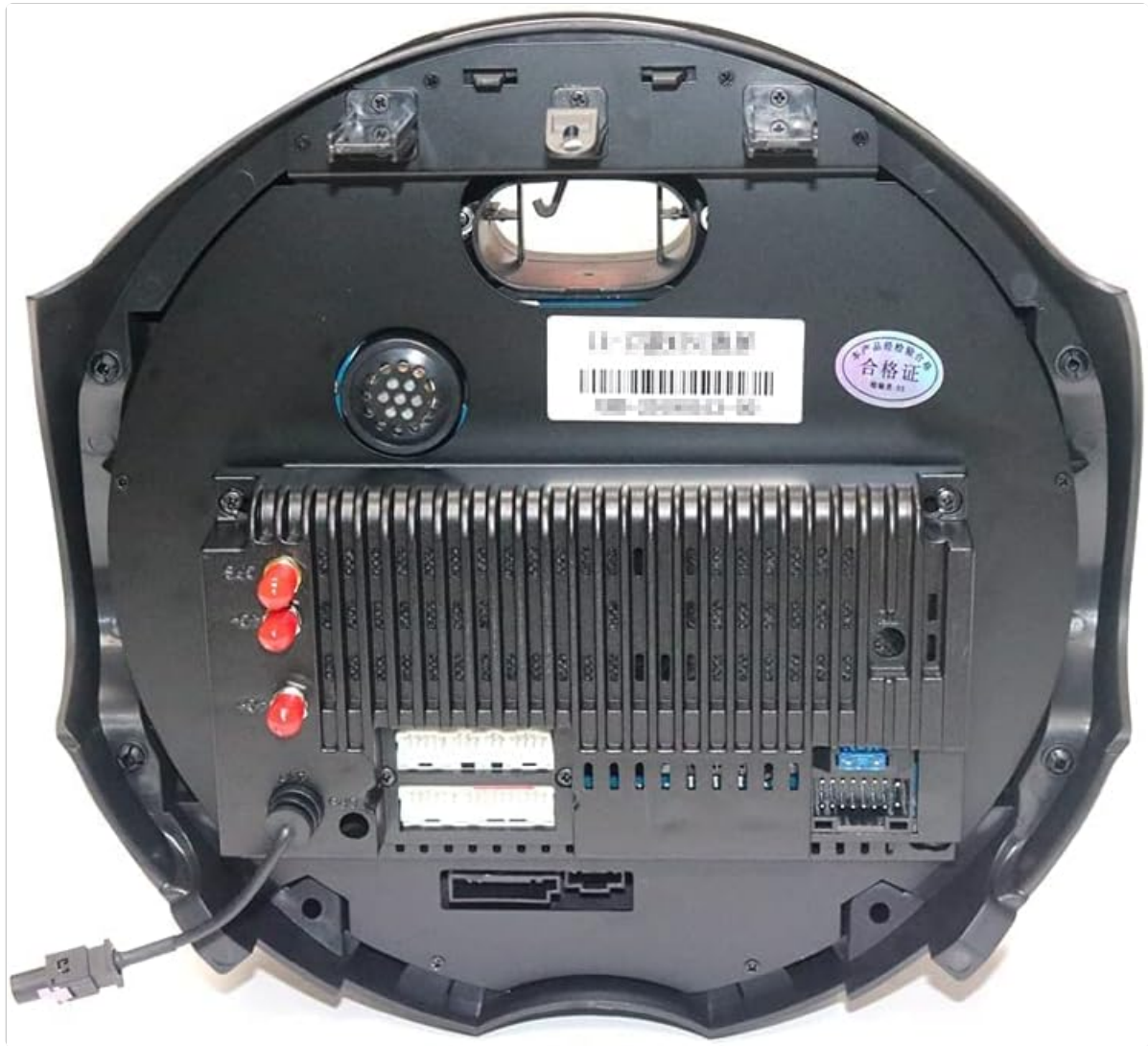
Image: Rear view of the KUNFINE car navigation stereo. This image highlights the various input and output ports on the back of the unit, including power, USB, GPS, and audio/video connections, crucial for installation.
