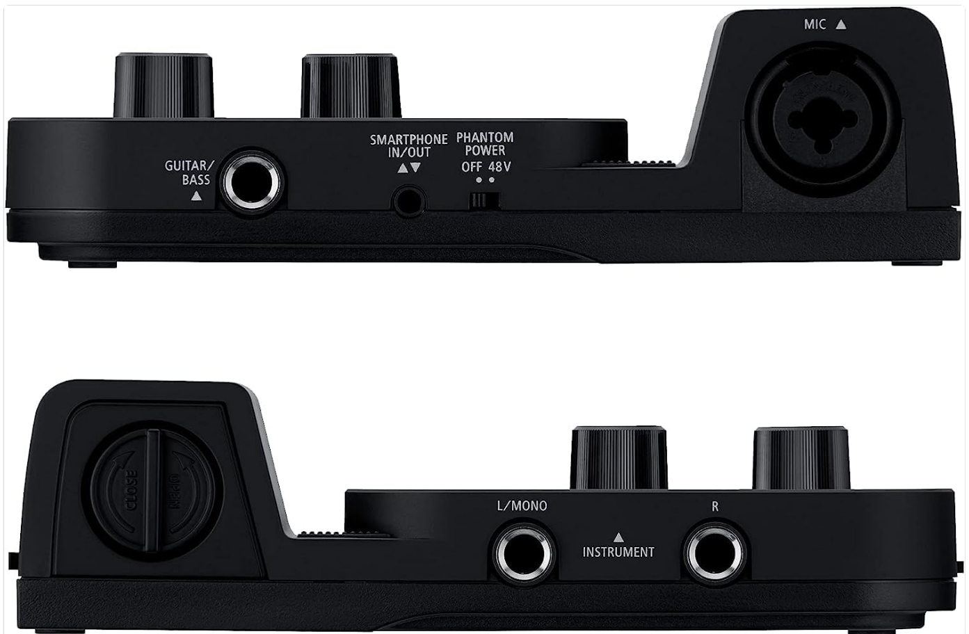
Image: Two side views of the GO:MIXER PRO-X. The top view shows the guitar/bass input, smartphone in/out, and XLR mic input. The bottom view shows the L/MONO and R instrument inputs.
