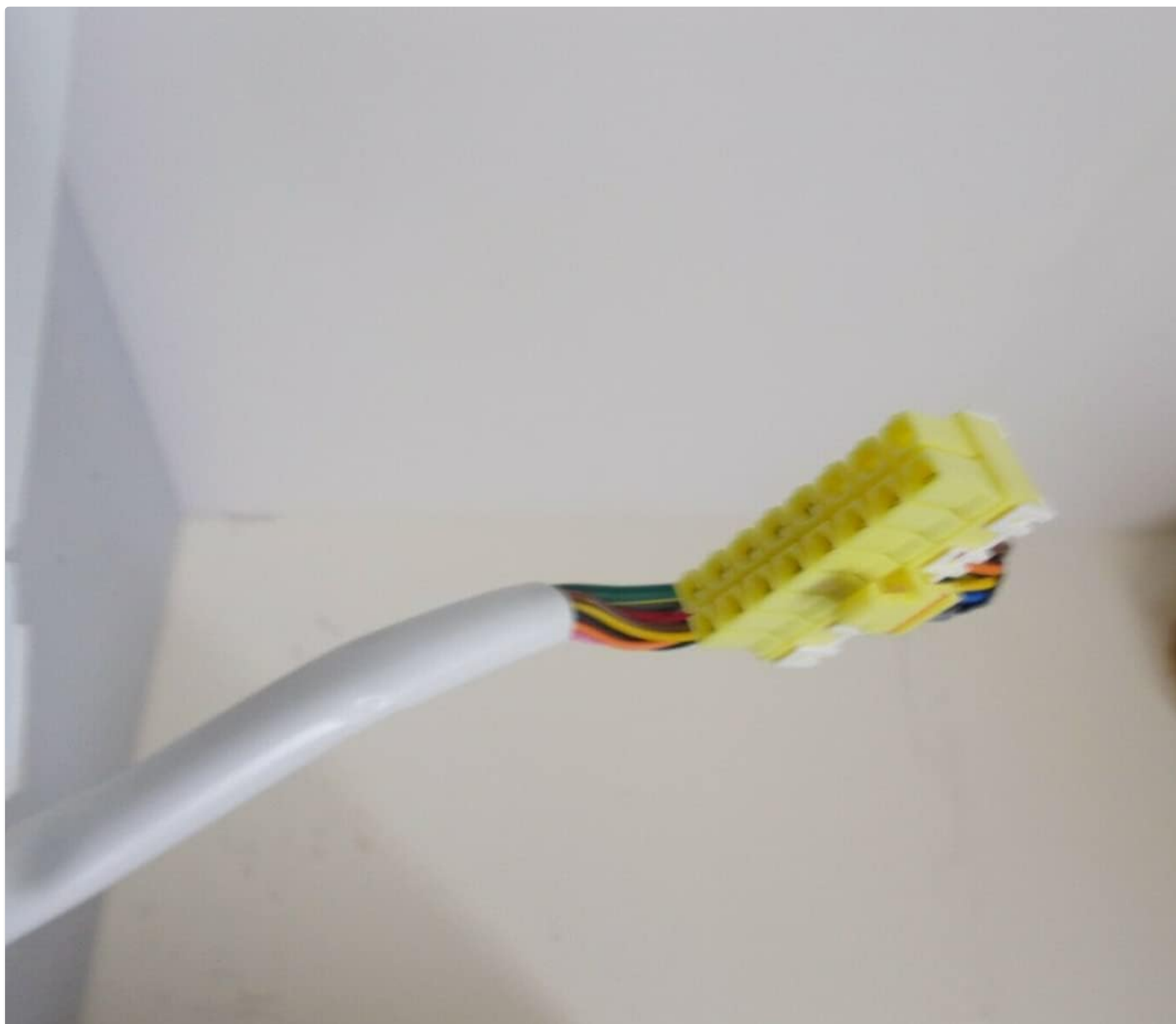
Figure 3.4: Detailed view of the yellow electrical connector, which connects the ice maker to the refrigerator's wiring harness.
