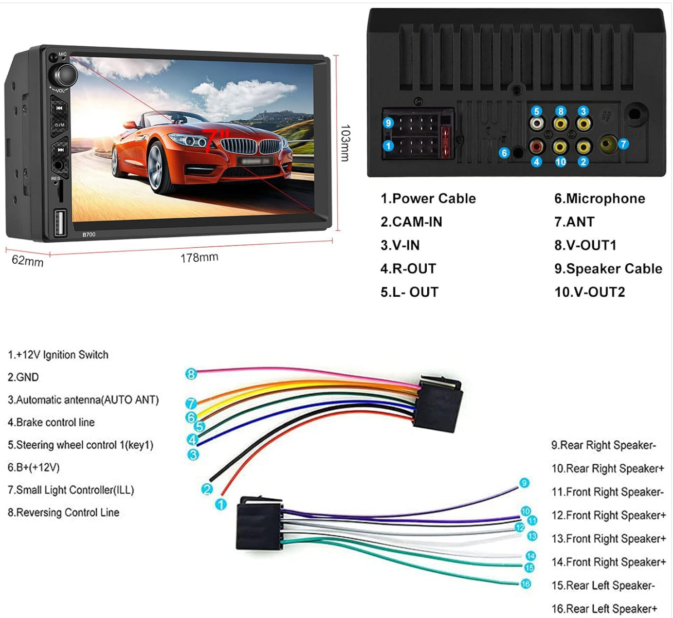
Image: Diagram showing the physical dimensions of the car stereo head unit. The unit measures 178mm in width, 103mm in height, and 62mm in depth.
