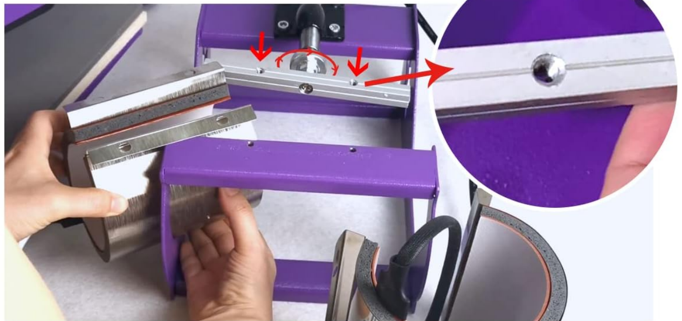
Image 5.2: Illustrations showing the updated thumb screw type mug press design for easy attachment and how to change the mug press attachment by unscrewing and sliding it off.
