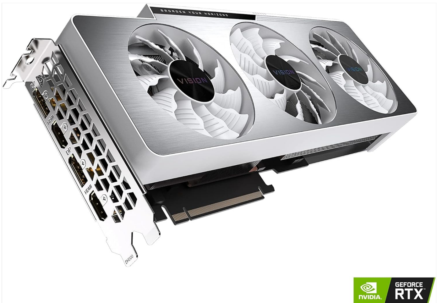
Image 4.1: Graphics card showing PCIe connector and display outputs.
