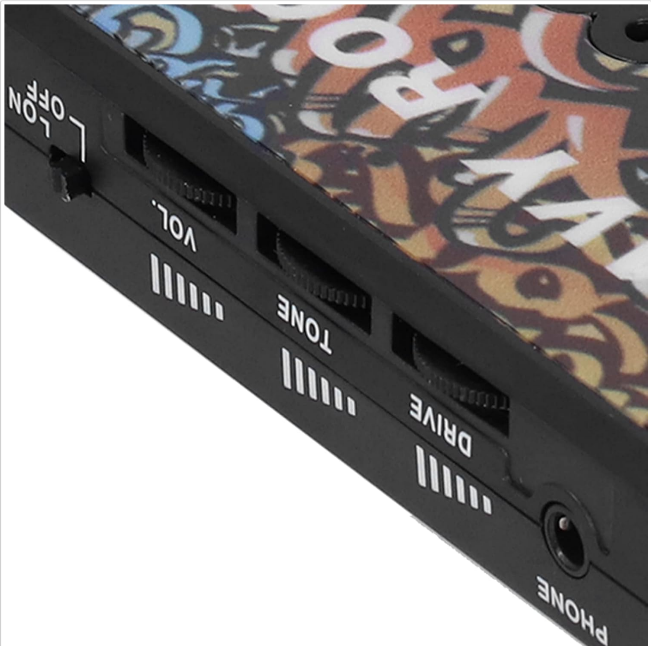
Figure 2: Close-up of the amplifier's control knobs: ON/OFF switch, Volume (VOL), Tone (TONE), Drive (DRIVE), and Headphone (PHONE) jack.
