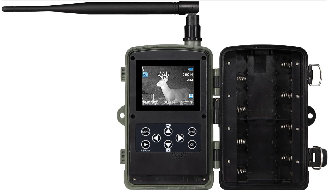
Figure 2: The camera opened, displaying the internal screen, control buttons, and the battery compartment on the right side.
