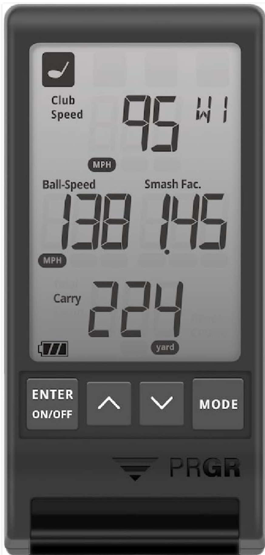
Figure 1: Front view of the PRGR HS 130-A displaying club speed, ball speed, smash factor, and carry distance.
