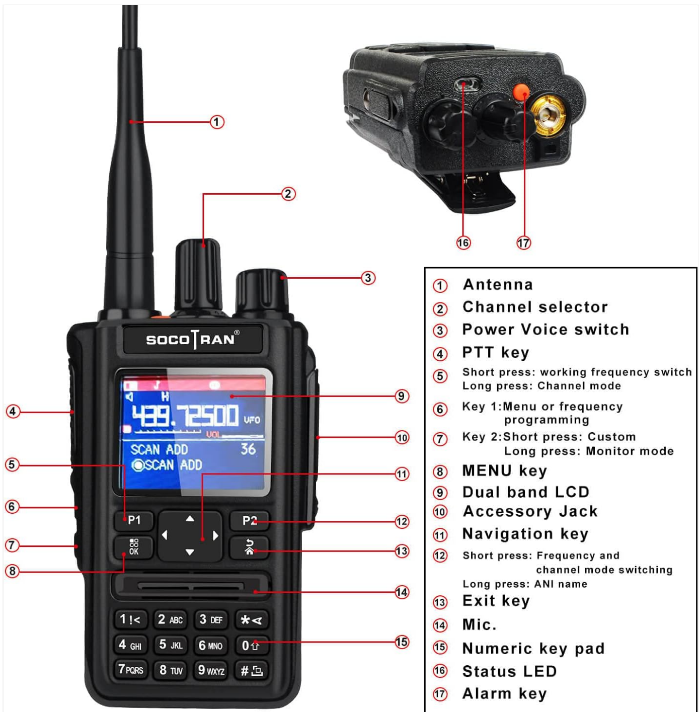
Figure 2: Labeled diagram of the JC-8629 radio components.
