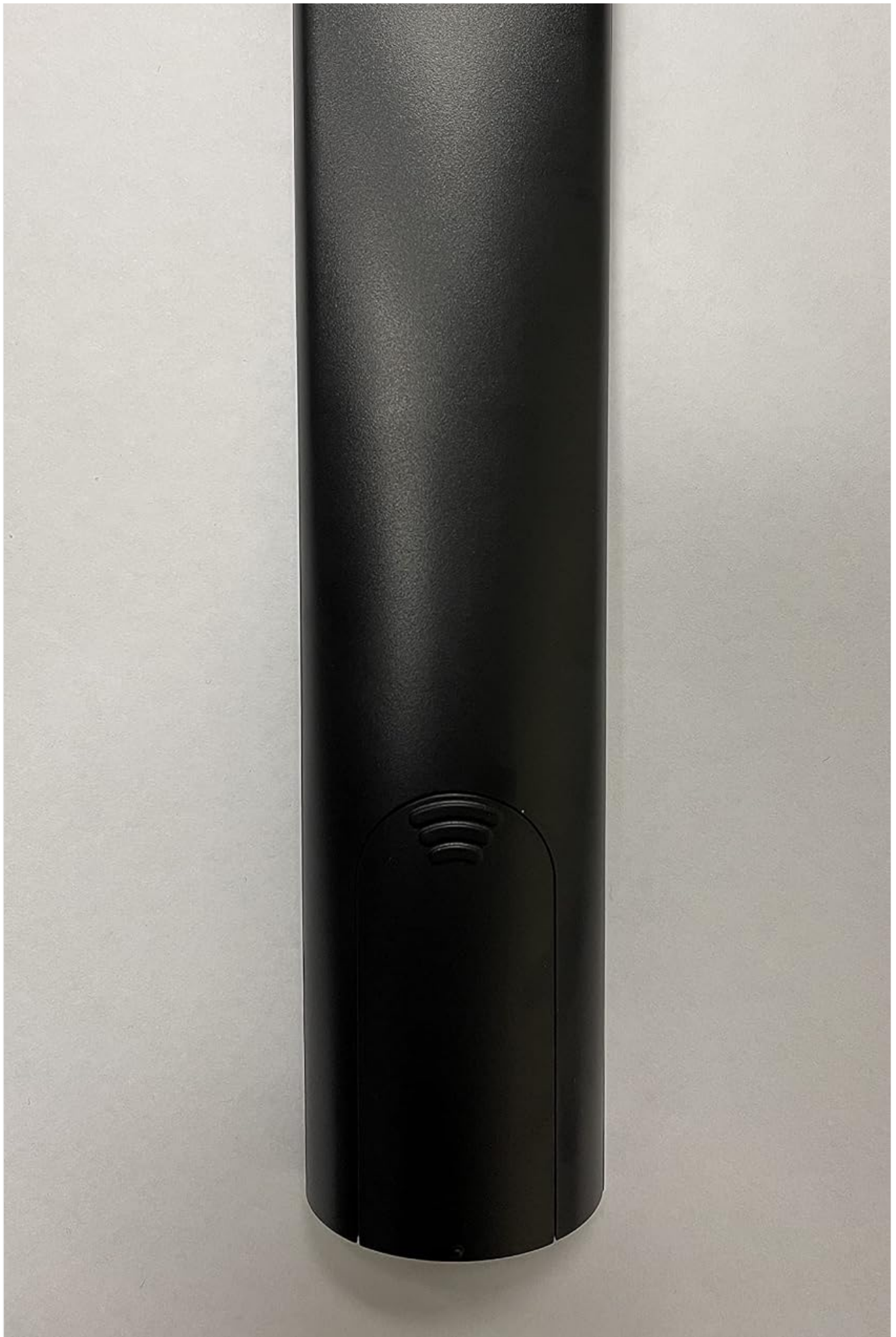
Figure 2.2: Back view of the USARMT 8142026670099K Remote Control. This image illustrates the rear casing of the remote, highlighting the battery compartment cover located at the bottom.
