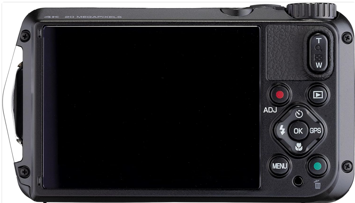
Figure 4.2: Rear view of the Ricoh WG-7, showing the LCD screen and playback controls.
