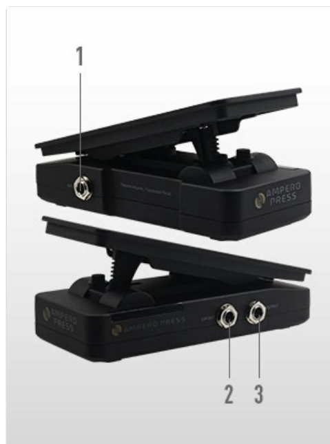
Figure 2.2: Side view of the Ampero Press SP30, highlighting the input and output jacks.
