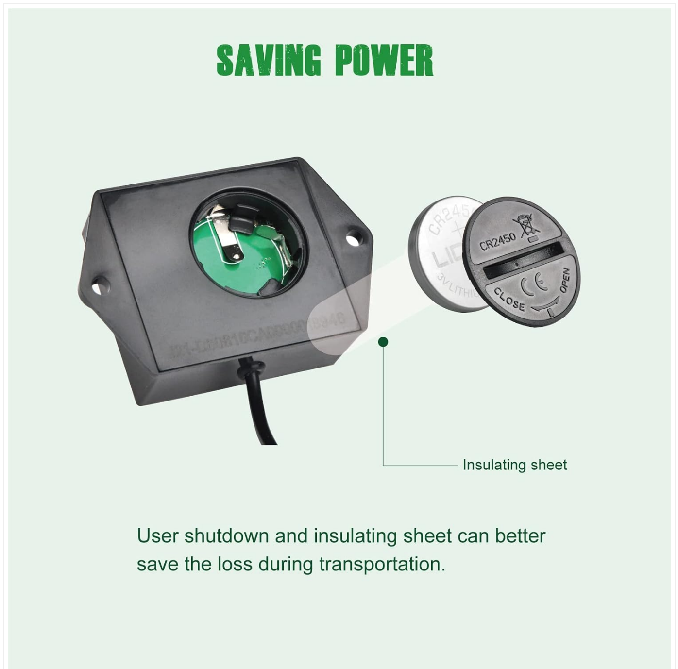
Figure 9: Power saving features. This image illustrates the CR2450 battery compartment and the insulating sheet, which helps preserve battery life during storage and transport.
