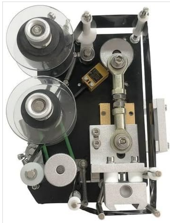
Figure 4.3: Top-down view of the label and ribbon loading area. This image details the label roll spindles, the ribbon spools for the date printer, and the various guides and tensioners that ensure smooth material feeding.
