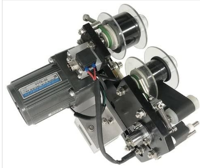
Figure 4.1: Main view of the YOU LIAN MT-130 Automatic Labeling Machine. This image displays the primary motor and the label dispensing mechanism, highlighting the robust construction of the unit.
