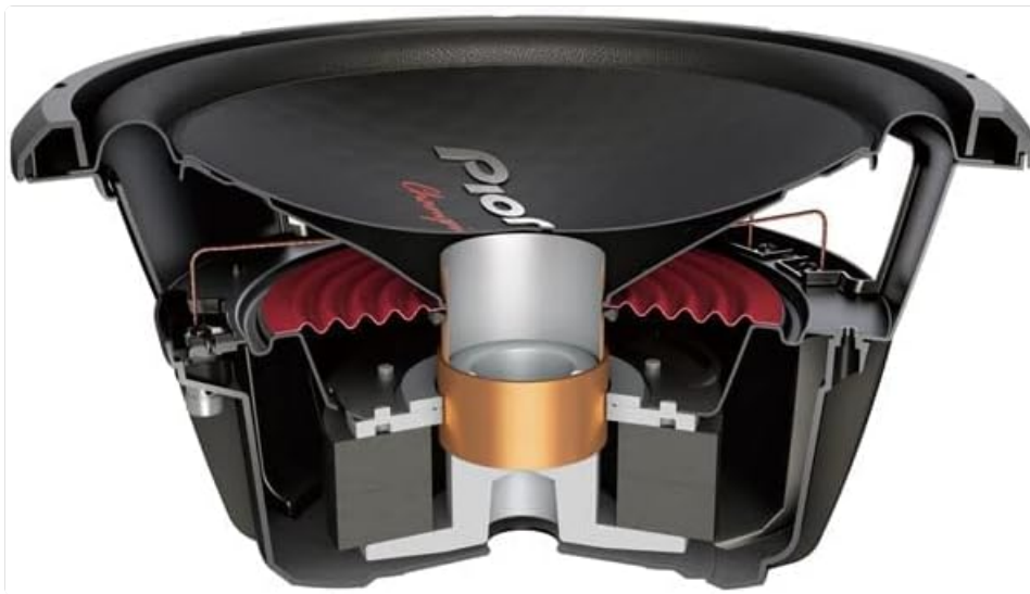
Figure 5.2: Cross-section view of the Pioneer TS-W312S4 Subwoofer, highlighting the voice coil, magnet structure, and cone assembly, which are critical for understanding its performance and wiring points.
