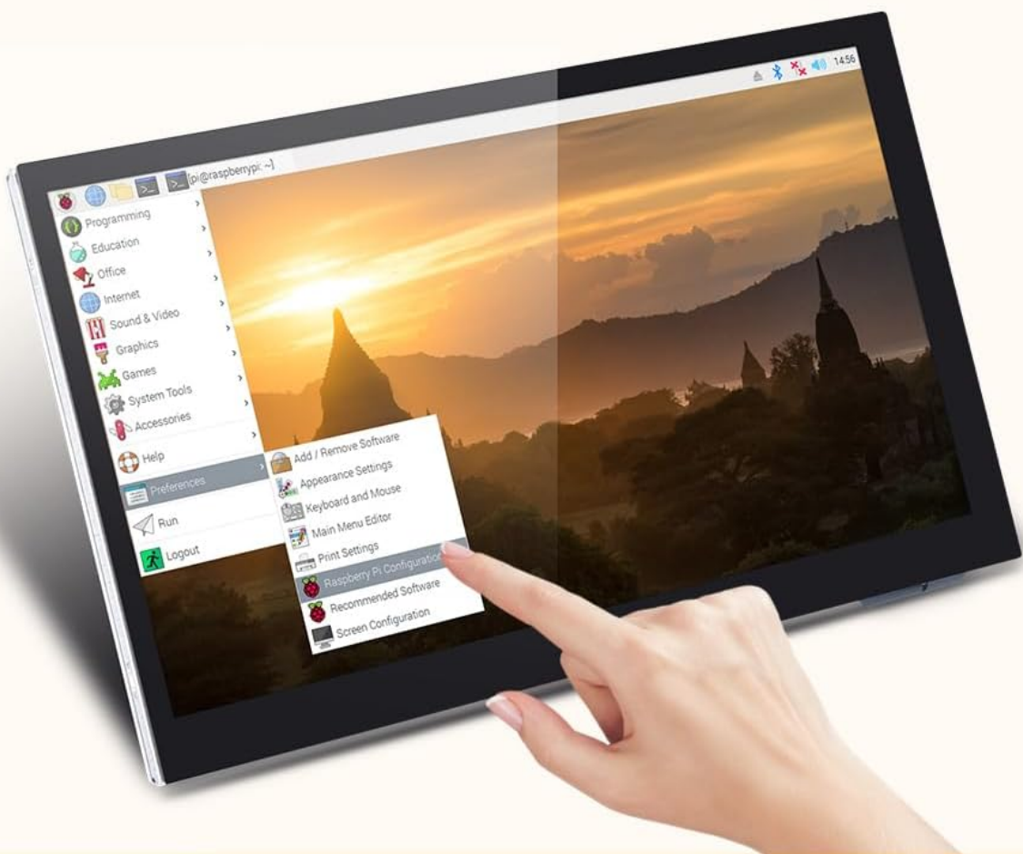
Figure 6: The 7-inch capacitive touch screen offers responsive and accurate touch control for navigating the Raspberry Pi's interface.
