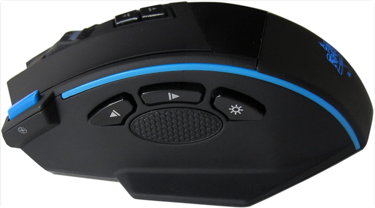
Image 3.1: Side view of the mouse, illustrating the placement of the forward, back, and light control buttons.
