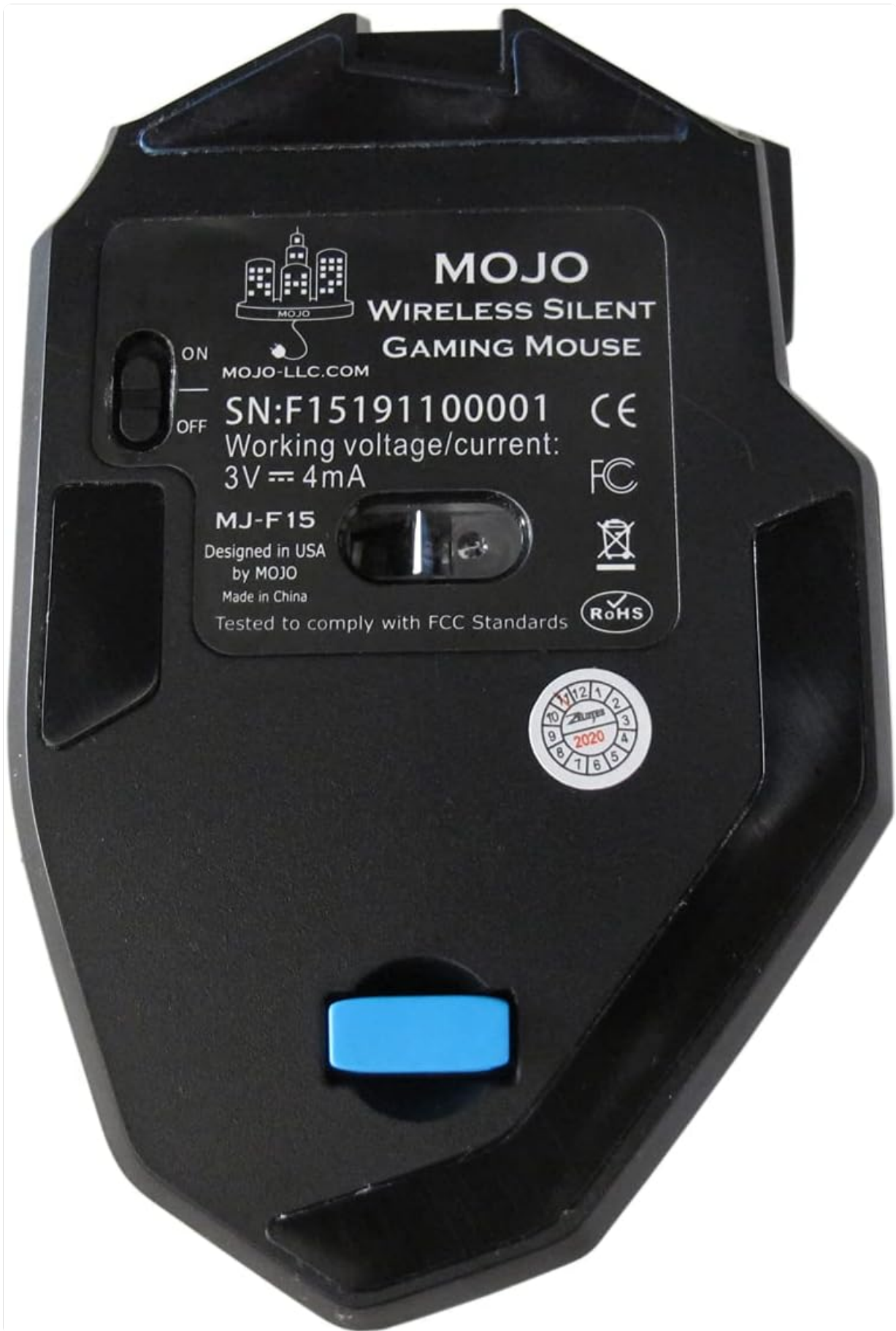
Image 4.1: Bottom view of the mouse, showing the optical sensor, power switch, and product label.
