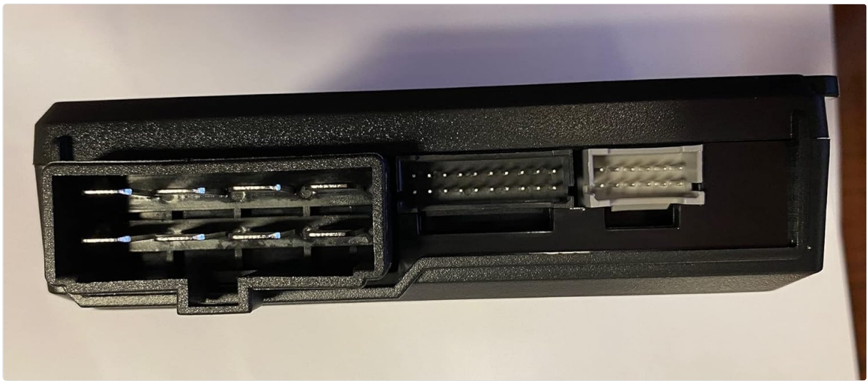
Figure 2: Side view of the Compustar CM-900 module. This image highlights the various input/output connector ports on one side of the module, where wiring harnesses are connected.
